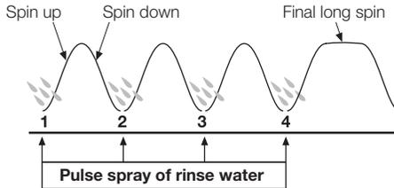
The machine will go through a series of **maximum** four pulse spray and short spin cycles in this manner, **depending on program selection**, followed by a final long spin that removes the water from the clothes to complete the full wash program.
